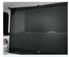
Net partition for luggage. The useful net partition offers security and protection from moving luggage. It's easily positioned within locating points in 'B' and 'D' pillars.
